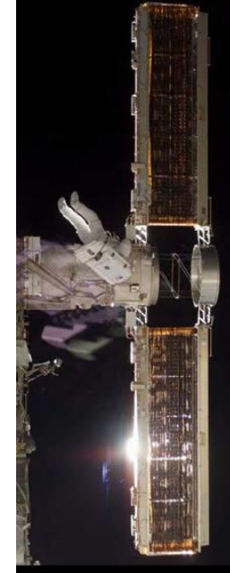
Astronaut releasing the fiberglass rods with drill
