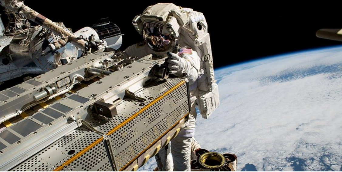
Astronaut unlatching the boxes containing the solar panels
