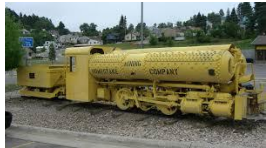
Compressed air trains used in mining operations to minimize chances of fires and explosions
