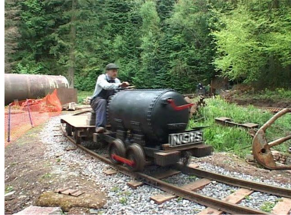
Compressed air trains used in mining operations to minimize chances of fires and explosions
