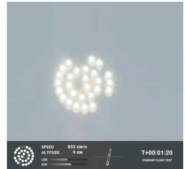
Engines on Space X Starship 1 damaged due to launch pad debris
