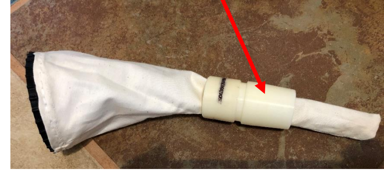
Hose filter bag with locking ring sewn
