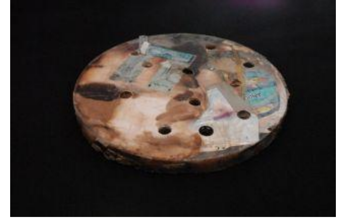
Plastic food packages, with some visible food residue, melted into a circular, plastic puck for potential use as radiation protection.
