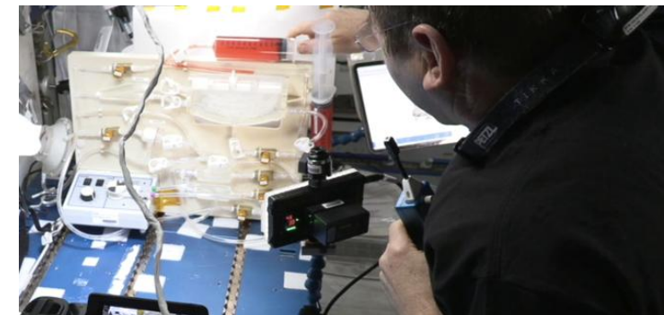
Above: Astronaut Mike Barratt Primes PWM-5 with test fluid.
