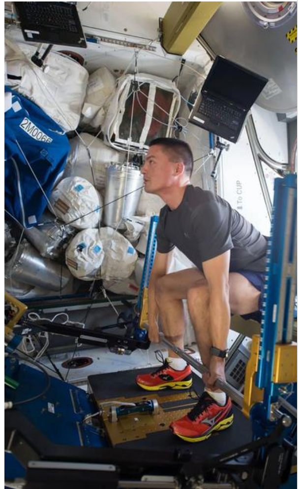
Photo B: NASA astronaut Kjell Lindgren performing a deadlift on the ARED aboard the ISS (Expedition 44, 2015). Note the foot anchor platform, blue frame uprights, and laptop used to log exercise data.
