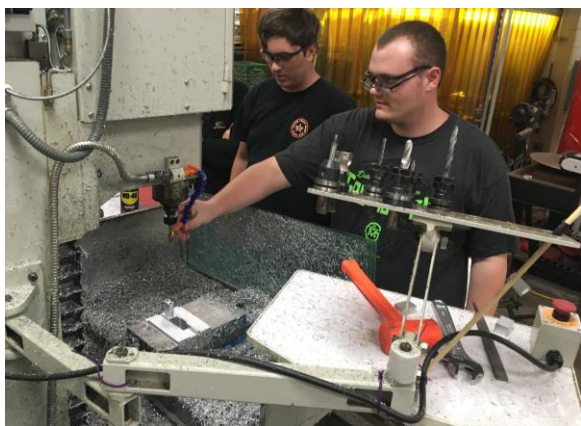
Roy Bellard works with students at Cypress Woods High School to run the milling machines that cut the parts. They use MasterCAM software with multi axis HAAS machines to make parts that are accurate to .005 inches and better.
