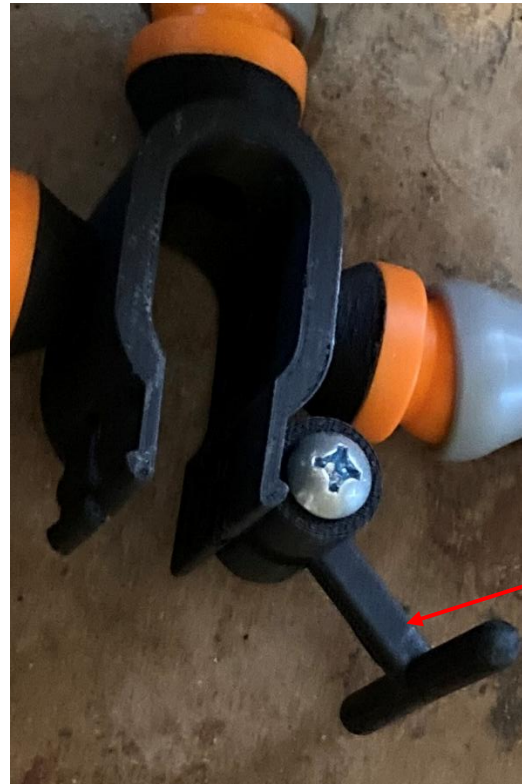
T-bar for latching onto handrail
