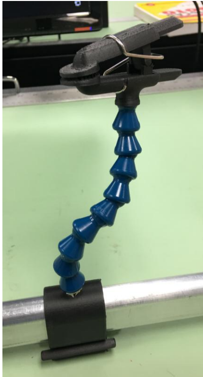
Main clip (black) slips onto the ISS handrails. 1/4" Lock line (blue) allows infinite positioning of the chip clip on top. The chip clip can hold onto many objects—gravity or not.
