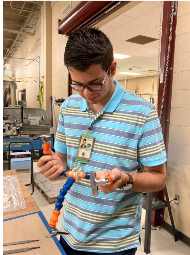
College intern Logan Sammons inspects final assembly with the printed ULTEM handrail clip. He helped make improvements on the design for easier assembly, preventing screws from scratching the handrails and final drawings.
