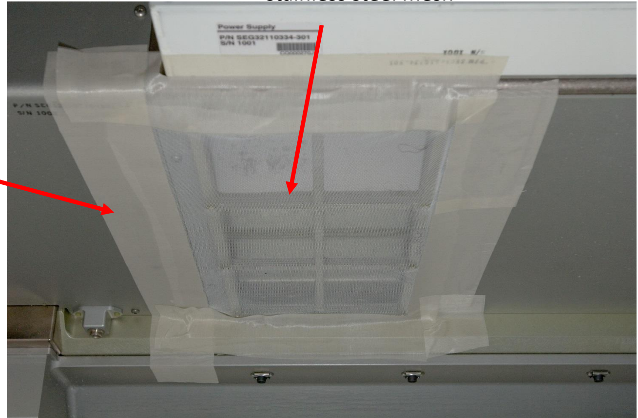
Grill is riveted onto the close out panel.
