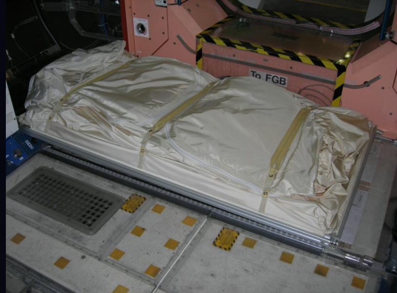
Flies up flat. Opens kind of like a pop-up tent. Rotates up from the bottom into the rack bay.
